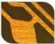
Short before Repair
