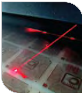
Using the mouse or keyboard arrows, a laser pointer is guided in seconds to locate and point to the defect's mark
