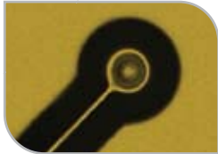
High accuracy registration results in imaging smaller annular rings
