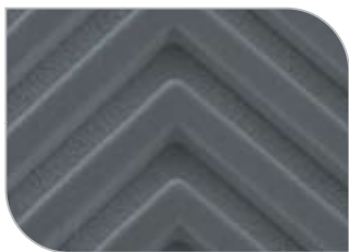
Fine lines down to 25µm/1mil for advanced HDI designs
